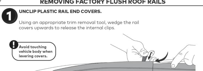
LIFT PLASTIC RAIL COVERS. Lift the outermost end of the front and rear covers up with caution. Lift outwards to avoid damage to rail
